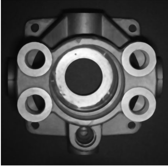
■ Fig. 14.24 Median filter, based on an 11 \times 11 pixel window. [ mdf(11) ]
