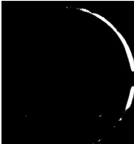
■ Fig. 28.11 Binarized image of part that has not been broached
