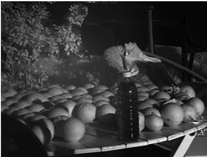
Fig. 10.16 Near infrared image taken using a CMOS sensor in sunlight through a 1,064 nm filter
