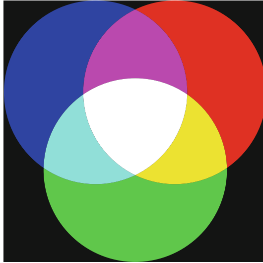
■ Fig. 4.24 Additive mixing of RGB primaries
