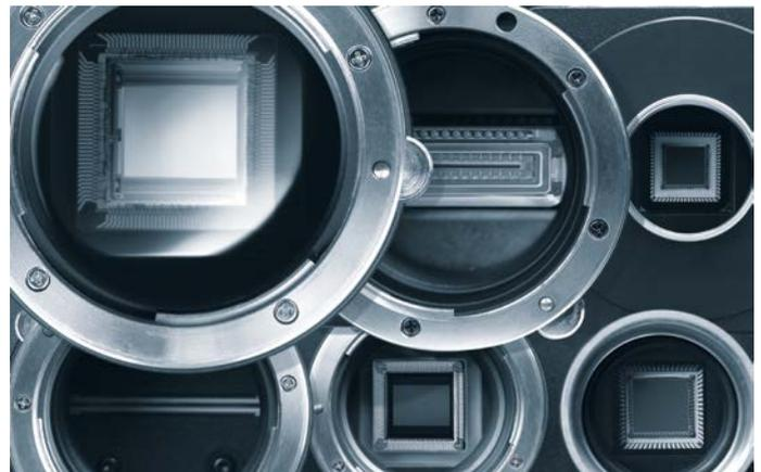
*View of the sensor of various cameras (top: area scan, line scan, area scan sensor; bottom: line scan, area scan, area scan sensor).*
